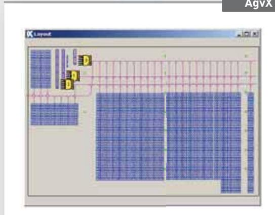
AgvX is able to handle any type of system, regardless of the quantity of nodes, their arrangement and the amount of AGVs. The software does not require any ad-hoc modification, but only by changing its configuration files, easily done by a specific graphics editor (Paths Editor).
